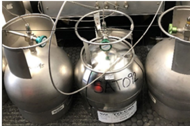
Figure 2: Example of Air Toxics Monitoring Equipment
