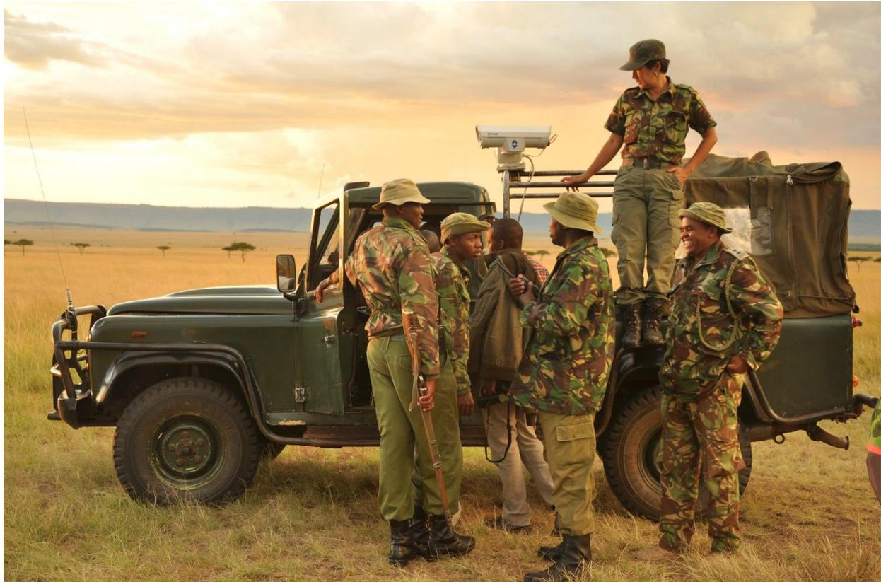
Fig. 3. FLIR thermal video camera mounted on a Mara Conservancy rangers' vehicle. The camera is connected to a video screen and joystick to enable panning of the open Mara landscape in search of poachers.
