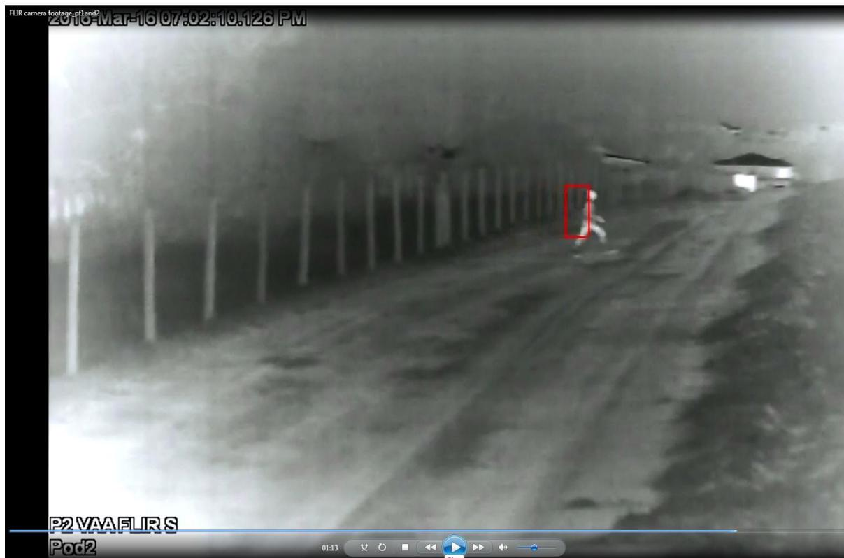
Fig. 2. FLIR thermal video camera system, with Avigilon human detection software in use in Kenya. The red box indicates that the cameras identified the object as a human and an alert was sent to rangers of an intrusion. The fence line to the left represents the perimeter of the park, with the road and right side of the image being inside the park.
