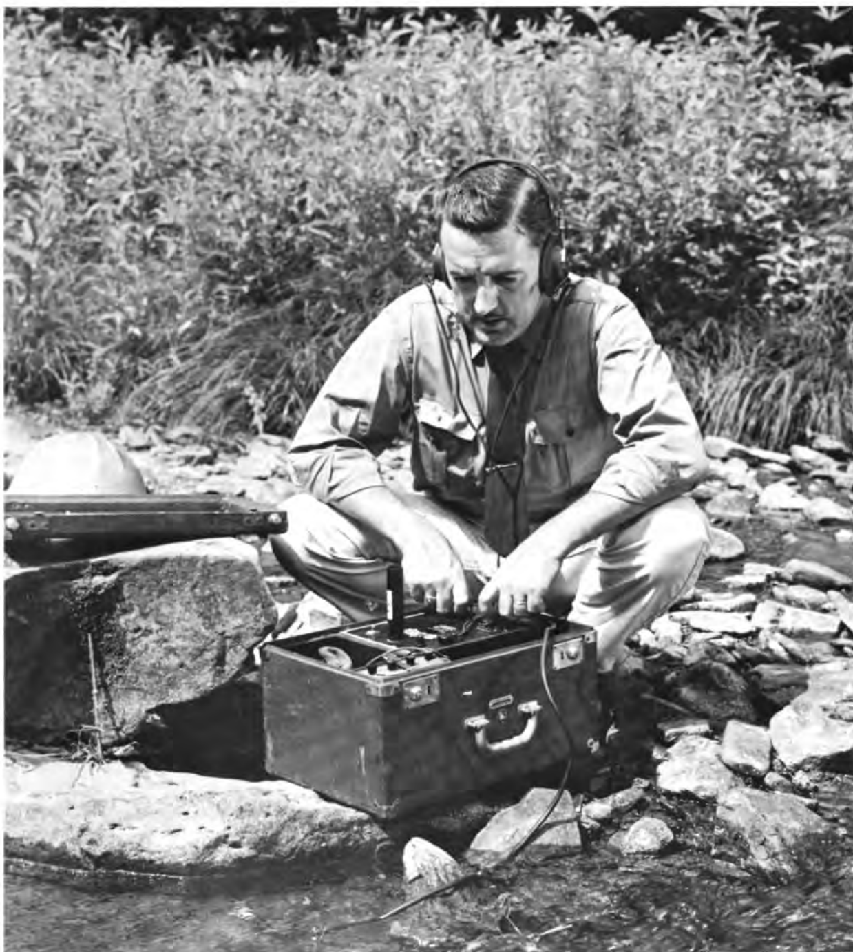
Measuring salinity of stream helps assess adverse effects of mining operation
