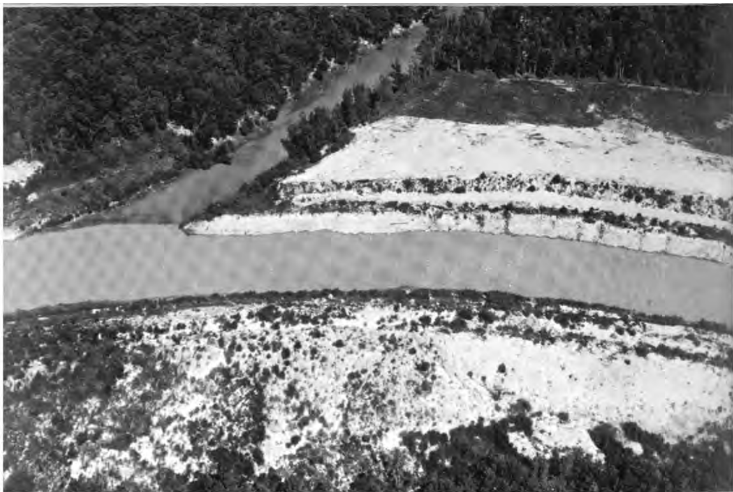
This picture of the junction of the "old" and "new" channel of the Forked Deer River in Tennessee illustrates effect of channelization on a natural environment
