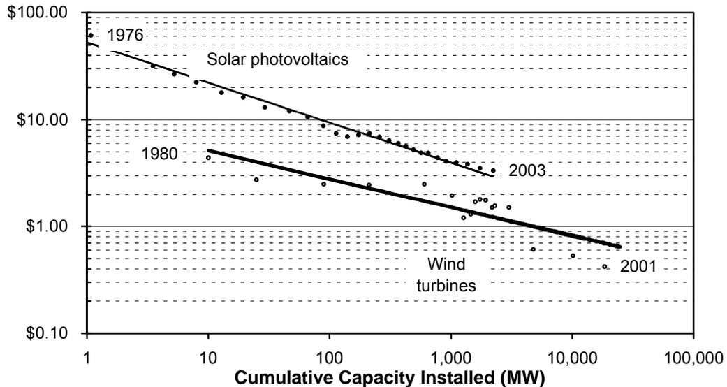
Figure 6: Capital costs of photovoltaics and wind turbines (constant 2004\$/Watt.) The horizontal axis shows cumulative worldwide installations of each technology (Duke and Kammen, 1999). Expanding production, driven by research, development, and deployment directly pays off in cost declines for the technology, and larger domestic markets further result in greater economic activity and job creation (Kammen, Kapadia, and Fripp, 2004).
